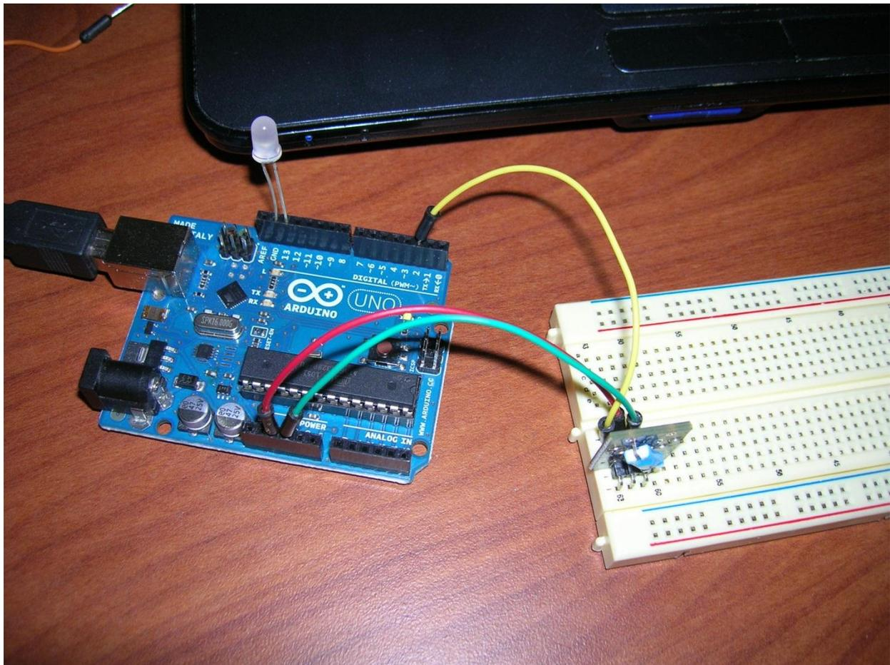
As always, take special care that you place the wires in the correct spots to avoid damaging the sensor. The ground wire should correspond with the pin near the – on the board. The Data wire should correspond with the pin near the S on the board. The 5V should correspond with the middle pin.
