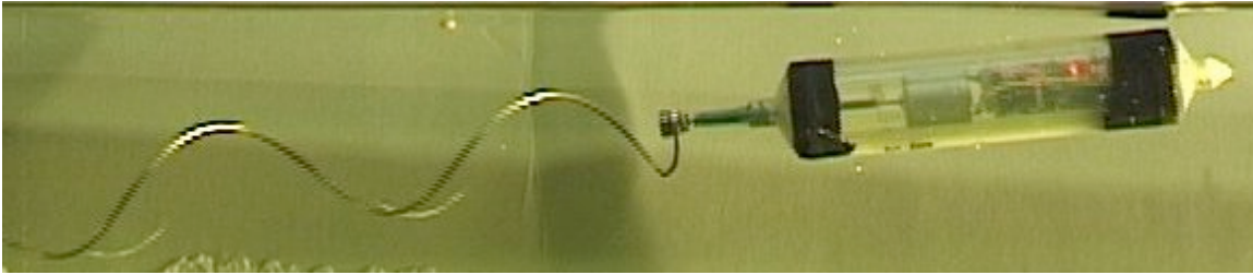
Figure 11. A low Re swimmer. For more information about it including detailed instruction on how to build it: http://students.washington.edu/ledel/LowRe/index.html
