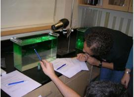
Despite strong 'wind' fluid from the upper layer does not mix much with lower layer fluid due to the density contrast between them (while mixing well within the upper layer). When no density contrast is present mixing occurs throughout the tank.
