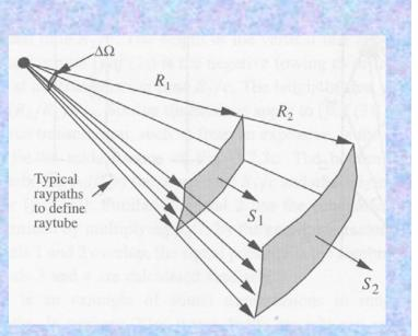
Ray propagation in a lossless refractive medium
