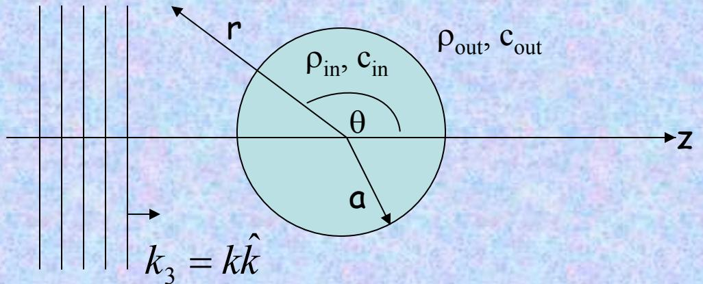
The problem is azimuthally symmetric, which facilitate its formulation in spherical coordinates.
