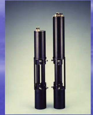
HOBi Labs Hydroscat-6: backscattering estimated from  $\langle\beta(140)\rangle$  at 6 wavelengths.
