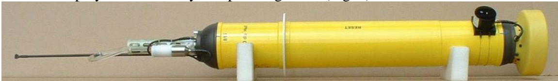
Figure 1. A profiling float float equipped with Conductivity temperature and depth sensor, oxygen sensor and the optical puck (the black sensor on the right-hand side). The integration of the optics into the float was the main thrust of this proposal.
