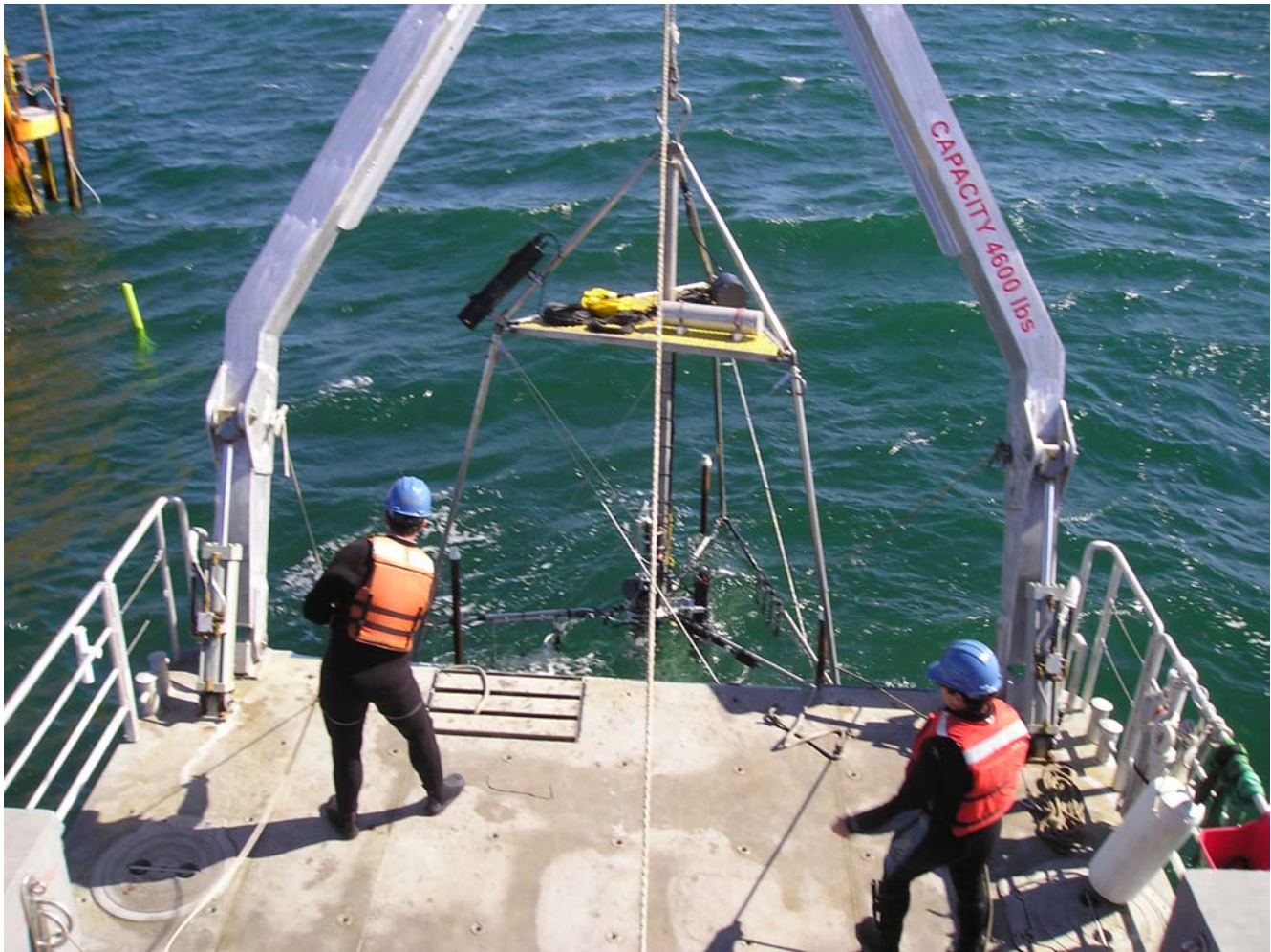
Deployment at the Optics, Acoustic and Stress in Situ (OASIS) tripod at the Martha's Vinyard Coastal Observatory on September 13, 2004. The TAPS (downward looking black cylinder) and data logger/manager are on the top of the tripod while most other instruments are 1mab.
