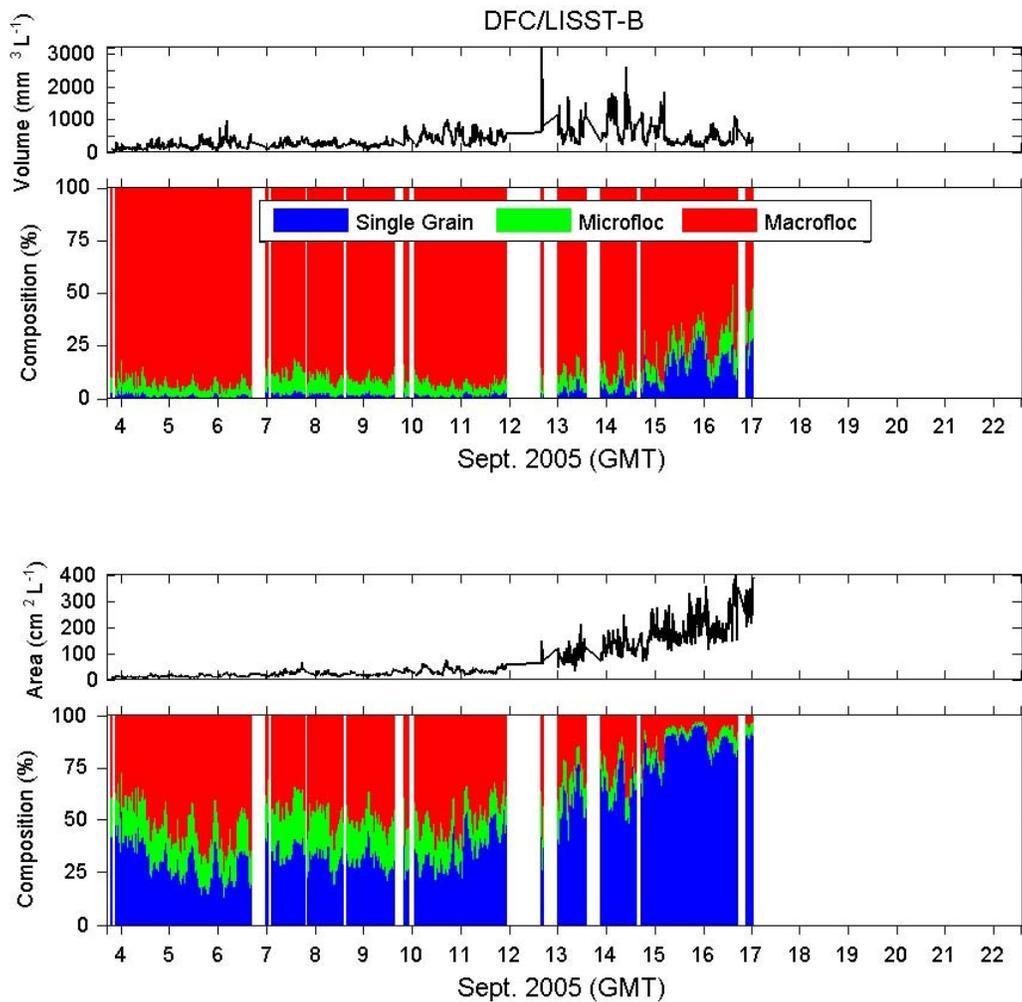
**Figure 4.** Volume concentration and area concentration (i.e. cross-sectional area) from the merged size distributions using the LISST-100 Type B and DFC apportioned into single grain (<36  $\mu\text{m}$  in diameter), microfloc (36 – 133  $\mu\text{m}$  in diameter), and macrofloc (>133  $\mu\text{m}$  in diameter) fractions. White regions represent periods of no data.
