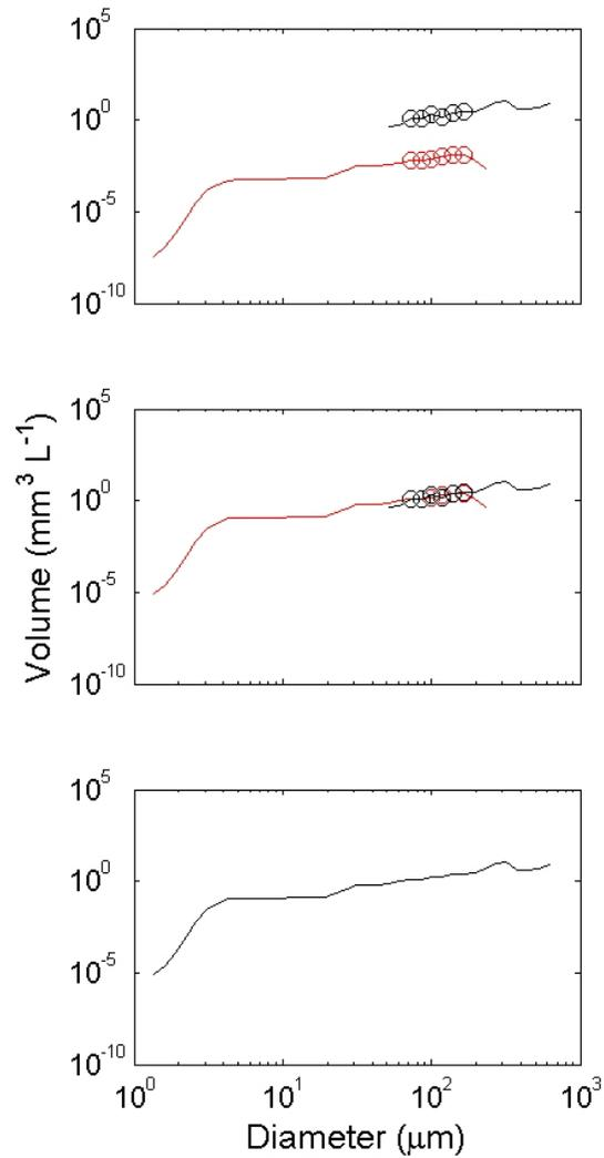
***Figure 3. Example of the LISST-100 Type B and DFC size distributions during adjustment that results in a merged size distribution 1.25  $\mu\text{m}$  – 1 cm in diameter. The red line represents the LISST-100 Type B size distribution and black line represents the DFC size distribution. The circles mark the region of overlap used for adjusting both size distributions. The adjustment factor for this data was 212. The data was collected on September 4, 2005, at 0444 GMT.***
