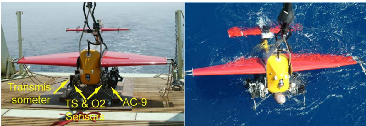
Figure 4. These pictures show the University of Washington Trisoarus tow vehicle equipped with the USC AC-9 absorption attenuation meter, beam transmissometer, chlorophyll and CDOM fluorometers, O 2 sensor, and physical sensors for T, C, and ADCP current profiling. This configuration was used in the Adriatic Sea for the Dolce Vita project.
