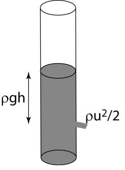
Potential energy, associated with the weight of the fluid above the hole is converted to kinetic energy of the fluid leaving the hole. The pressure at the hole is the atmospheric pressure  $(p_{atm})$ + the hydrostatic pressure:  $\rho gh+p_{atm}$ .
