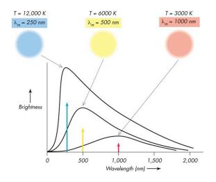
Every body radiates heat (energy) depending on its own temperature. The warmer it is the more it radiates and the shorter is the average wavelength it radiates at.
