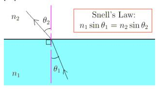
Shine a laser pointer into the center of the side of the water tank. Observe the angle change due to refraction.
