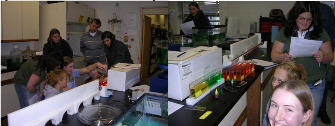
Caroline, Veronica, Amanda, Amber, Nick and Laura observe diffusion of colored fluids of the same density. It took a very long time for the color to homogenize (more than an hour).
