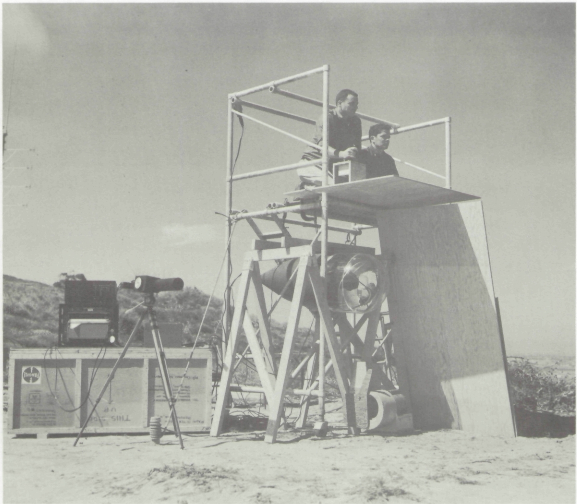
Figure 13. Searchlight mounted under scaffold, with two observers in position.
