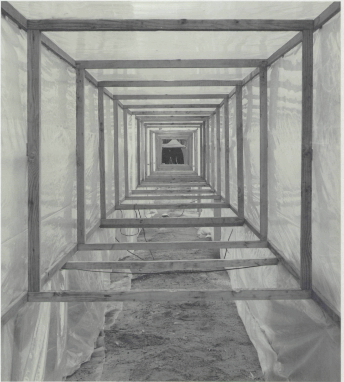
Figure 8. Photograph of the inside of the fog tunnel looking toward the autocollimating theodolite.
