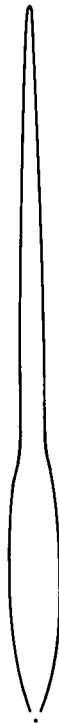
Fig. 46. Detection Lobe for Uniform Circular Object, Background Luminance 75 Ft-L, No Contrast Attenuation; 1/3 Second Fixation.
