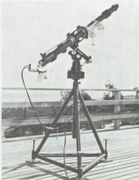
Fig. 21. Ground site tripod-mounted photoelectric photometer.
