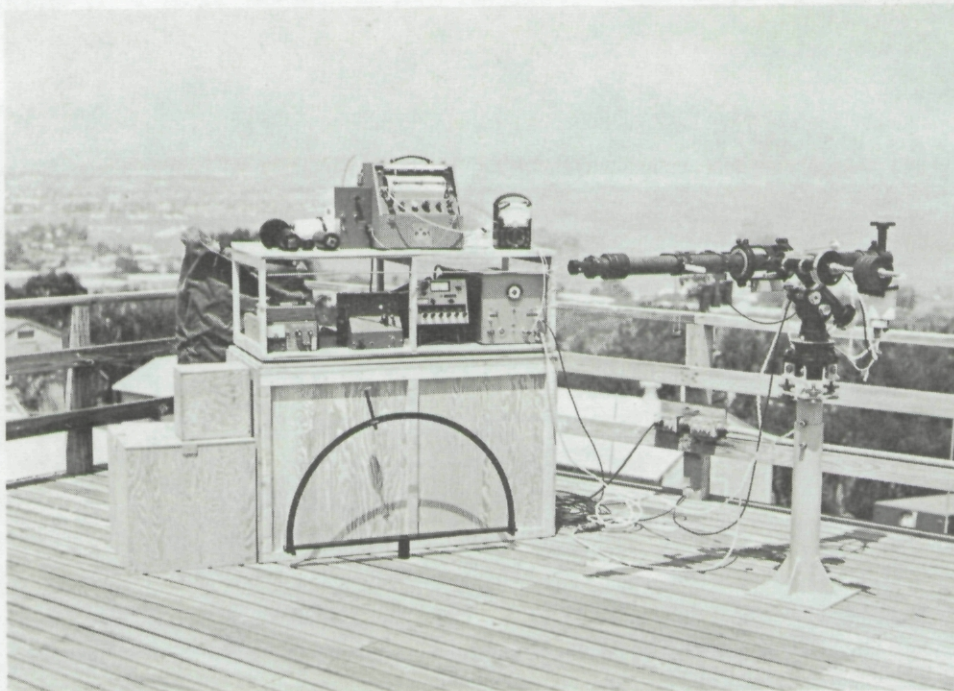
Fig. 22. Ground site photoelectric photometer with recording unit.
