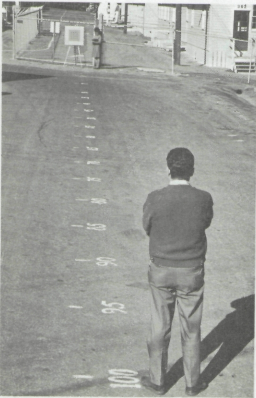
Fig. 2-1. Outdoor observing range at the Visibility Laboratory. The displays are scaled so that each foot on the range corresponds to one nautical mile of orbital altitude.
