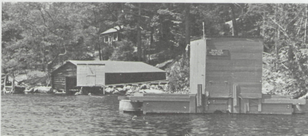
Fig. 2-10. Floating instrument platform (barge) moored near the outer end of the underwater track at Diamond Island. The laboratory building can be seen on the wooded slope beyond the boat house.
