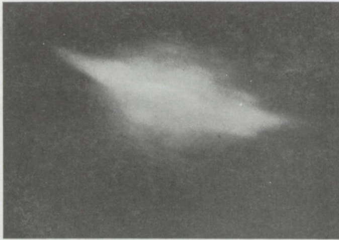
Fig. 6-2. Photograph of the beam pattern produced by a second harmonic green laser built by the Lear-Siegler Corporation. The KDP crystal was outside the resonant cavity, just as in the case of the 1966 RCA underwater laser.
