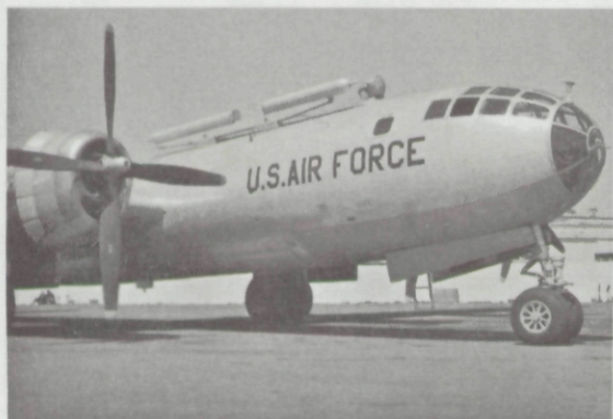
FIG. 3. Specially instrumented B-29 aircraft used to collect the data presented in this paper. The long cylindrical apparatus on top of the fuselage is the attenuation meter , shown schematically in Fig. 4. The smaller cylindrical device which appears slightly forward of the attenuation meter is the sky-scanning telephotometer. It consists of an end-on type multiplier phototube mounted at the focal point of a parabolic front-surfaced mirror 12 in. diam. Scanning is accomplished automatically by means of a turret and trunion mounting; scanning time for the entire hemisphere is 90 sec. Field of view, adjustable by means of interchangeable field stops, was circular, 5° in angular diameter in the case of the data shown in Fig. 6. Sensitivity is sufficient to map even the darkest high-altitude night skies. Spectral response is controlled by absorption filters. A similar (downward-viewing) telephotometer is mounted beneath the aircraft but is not shown by this photograph.
