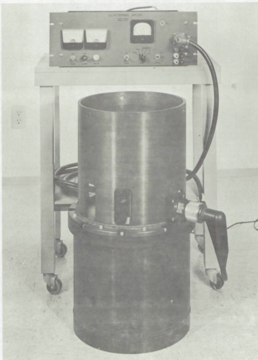
Figure 4. General Angle Scattering Meter.
