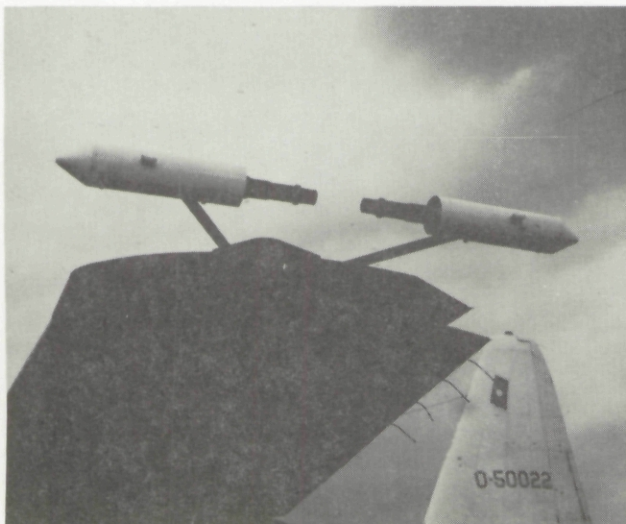
Fig. 3-4. Variable Path Function Meter.
