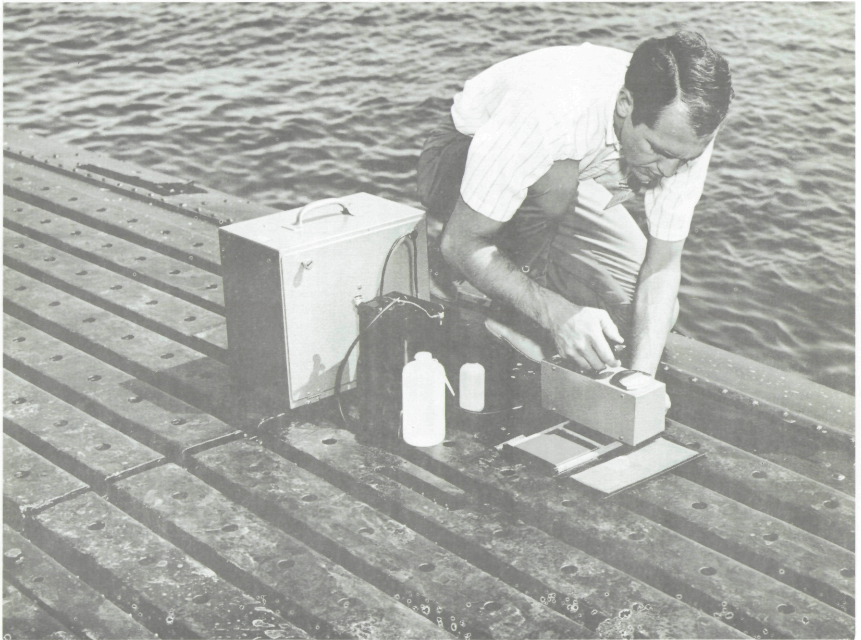
Fig. A-1. Gardner Laboratory 45°, 0° Portable Reflectometer with Visibility Laboratory Circuit Modifications Providing Increased Sensitivity for Low Reflectance Measurements
