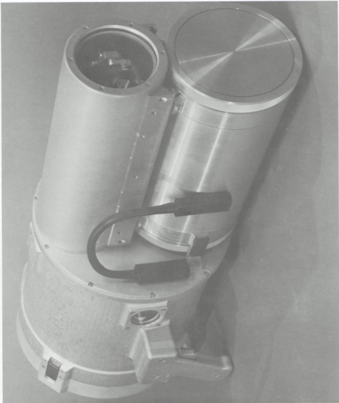
FIGURE 14. Photograph of underwater laser scanner unit in its underwater housing (compare with Figure 3). The laser beam exits through a 3/8" thick acrylic window. Below the laser housing is the larger diameter battery housing, which may be easily removed from the remainder of the underwater housing. A short cable, with underwater connectors, connects the underwater battery pack to the underwater housing. The exit port for the sync pulse flash lamp (one of two) can be seen on the side of the underwater housing. The underwater unit is carried by means of either or both of two handles. The handle which can be seen in the photograph contains the hand trigger for initiating a scan sequence.
