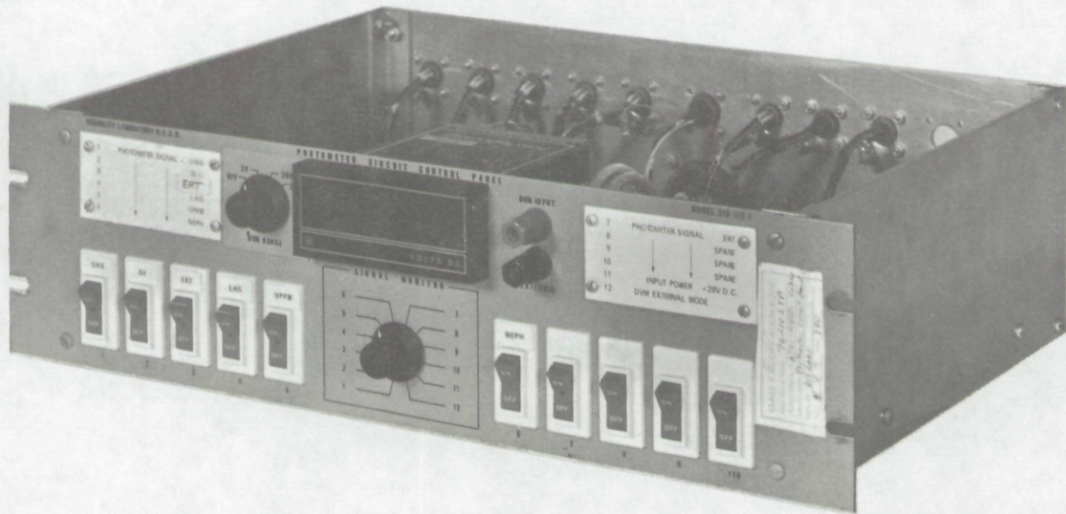
Fig. 3-6. Photometer Power Distribution and Readout Panel.
