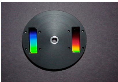
Figure 3. Filter wheel of ac-s.
