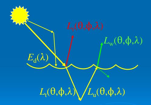
An instrument measures  $L_u$ (in air), but  $L_w$  is what tells us what is going on in the water. It isn't easy to figure out how much of  $L_u$  is due to  $L_w$ .
