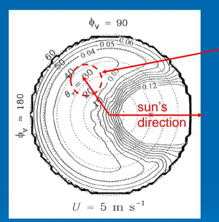
ρ as a function of polar and azimuthal viewing angles for a given sun zenith angle and wind speed an azimuthal viewing direction of roughly 135 degrees from the sun and 30-40 deg from the nadir is optimum for making measurements:
