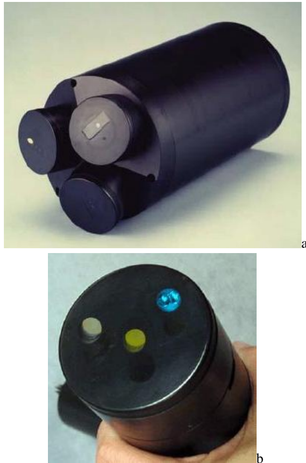
Figure 1.1. a) ECO-BB9 instrument showing the three BB3s. b) BB3 detail. Colored circles are LED sources and adjacent black circles are the corresponding detectors.
