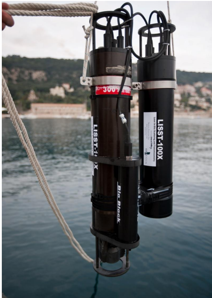
Figure 1: Lisst 100X (left) and his external battery (right) before deployment in Mediterranean Sea (Malika Kheireddine).
