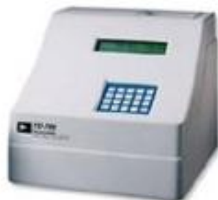
Fig. 4. TD-700 bench-top fluorometer (Turner Designs). 12x35 mm round screw top vials hold the samples, which are introduced inside the instrument for reading. A black plastic standard accompanies the instrument for necessary calibrations.
