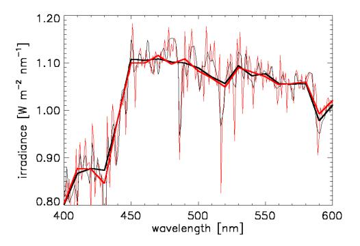
Fig. 2. Comparison of RADTRAN (black) and RADTRAN-X (red) total downwelling plane irradiances band averaged to 10 nm resolution (heavy lines overlying the 1 nm data of Fig. 1).
