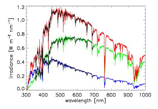
Fig. 3. RADTRAN-X computed values of the total (red), direct solar (green), and diffuse sky (blue) irradiances for the conditions of Fig. 1. RADTRAN values are overlaid in black for 350-700 nm.
