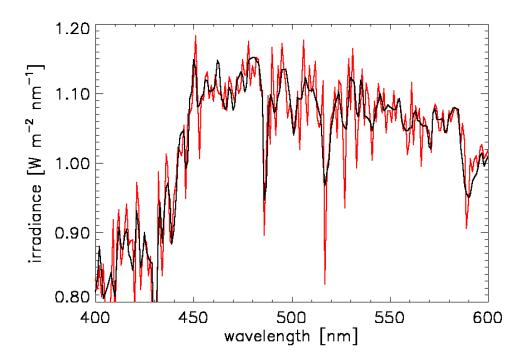
Fig. 1. Comparison of RADTRAN (black) and RADTRAN-X (red) total downwelling plane irradiances at 1 nm resolution for a particular set of atmospheric conditions.
