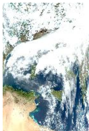
Figure 18.4: An RGB Image with Rayleigh Correction
