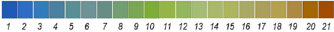
Fig. 1. Approximate colors of the Forel-Ule indices FU = 1 to FU = 21 (copied from Wernand and van der Woerd, 2010a).
