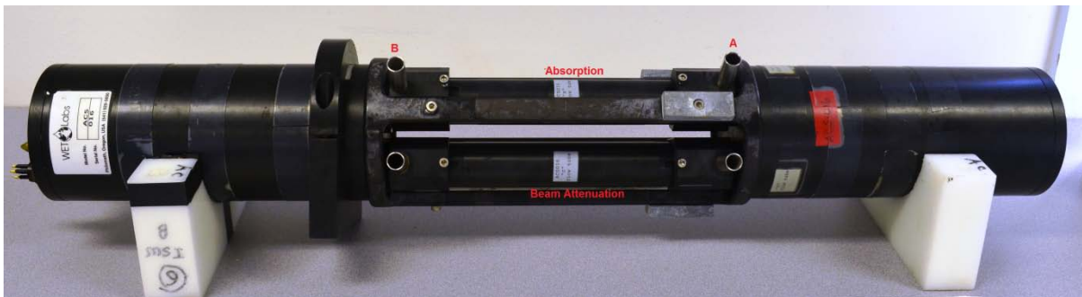
Figure 1 AC-S absorption and beam attenuation meter. The absorption and beam attenuation chambers both have flow inlet (A) and flow outlet (B). Note that these inlet and outlet can be reversed without changing measurement.
