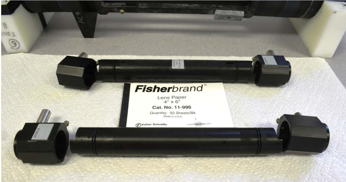
Figure 4 The AC-S 16 tubes and tube sleeves disassembled for cleaning using lens paper.
