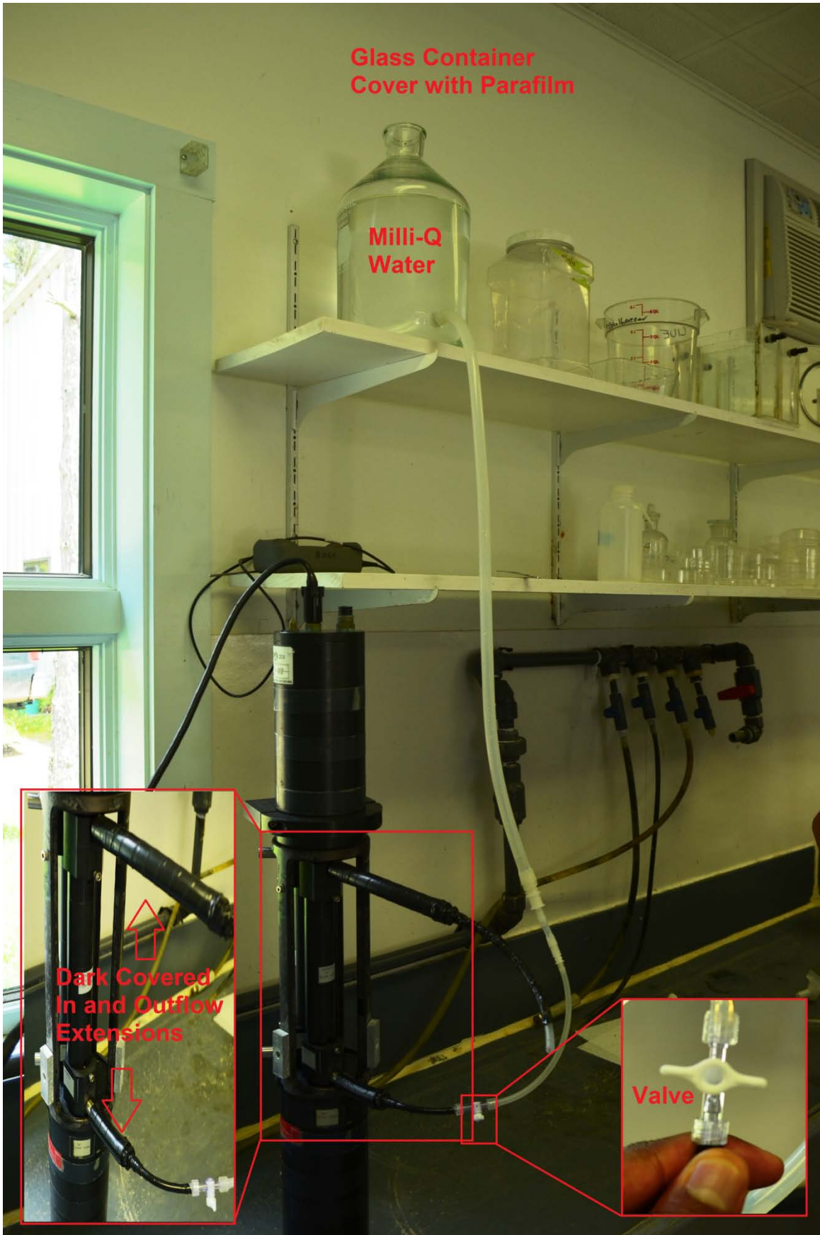
Figure 6 Illustration of setting up calibration components. Use dark tape covered inflow and outflow tubes, a valve to control water flow and elevated location for the glass container with Milli-Q water.
