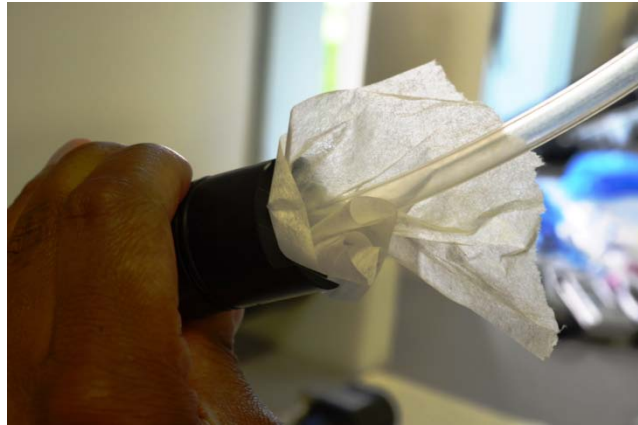
Figure 5 Steps in applying the isopropyl alcohol A , cleaning the sensor windows B , and tubes C .
