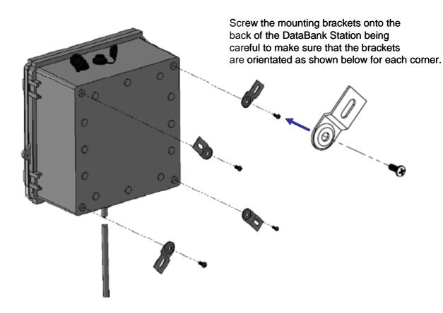
Note: The DataBank Station should NOT be mounted in direct sunlight and should be shaded.
