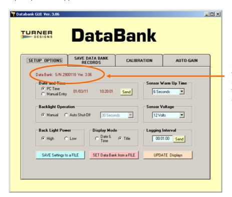
Upon connection, the DataBank's serial number and version of the operating system are displayed
