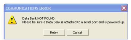
If you *click* Retry, then the GUI again tries to find the DataBank. If you *click* Cancel, then the GUI software will shut down and you must re-start the GUI. Once communication has been established, the main screen will display the DataBank's information in the upper left hand corner and the "*Talking with DataBank*" prompt will disappear:
