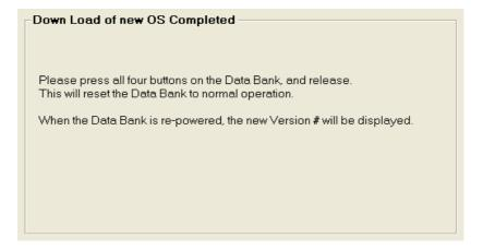
Simply follow the instructions in the window to reset the DataBank and return to normal operation.
