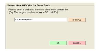
Note: Both of the methods for upgrading will result in the screen above. Click the Browse button to navigate to a valid Hex file. Valid Hex files begin with a DB and end with (.hex) and contain the operating system's version within the filename. For example, <u>DB3xx.hex</u> is a valid Hex file that can be used to update the DataBank's operating system to version 3.xx
