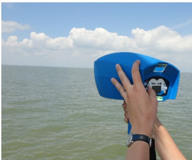
Figure 5: Correct positioning of the WISP-3 during the measurement
