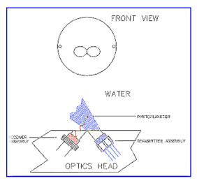
reject the small amount of out-of-band light emitted by the LED. The light from the source enters the water volume at an angle; in the figure to right, the angle is approximately 55–
