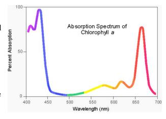
Chlorophyll *a* absorbs in both blue (Soret) and red (Q) bands (figure; source is <a href="http://www.ch.ic.ac.uk/local/projects/steer/chloro.htm">http://www.ch.ic.ac.uk/local/projects/steer/chloro.htm</a>). Chlorophyll *a* has the additional characteristic of fluorescence, a phenomenon by which a fraction of the photons are re-
