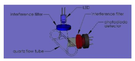
well in a ship's in-line systems. The source and detector are at 90° to each other (see figure below). Note that if a sample is kept within the flow tube for too long the fluorescence of the sample will change due to the exposure to light.
