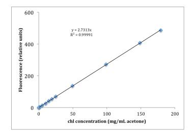
Fluorometer calibration with pure chlorophyll a standard
