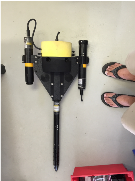
Hyperpro in TSRB mode (Tethered Surface Radiometer Buoy)
