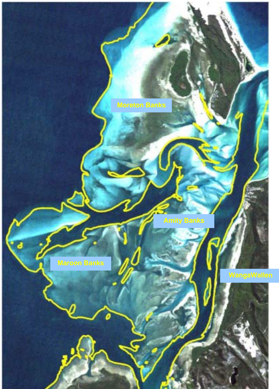
Figure 11. Image mask outlines overlaid on the August 2004 image. Yellow = 3.0 m AHD bathymetric contour. The mask was used to exclude select areas for image processing operations.
