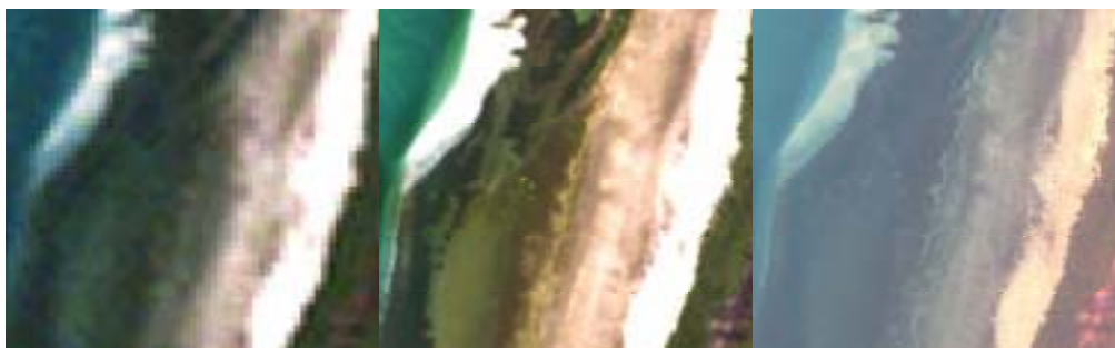
Figure 10. Example of the spatial resolution differences for the image data sets collected over a 1.5 km x 1.5 km area of the Wanga Wallen Banks. From left to right: Landsat 5 TM (30 m), CASI-2 (4 m) and Quickbird-2 (2.4 m).
