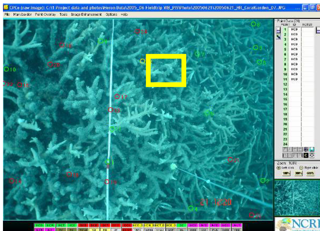
Figure 7. Screen grab of photo analysis CPCE program. Main photo with circles in different colours (green = class assigned, red = class not assigned yet, yellow = class currently assigned). On the right is table with point numbers and its assigned classes. On the bottom the coloured bar represents the different class types that can be assigned.
