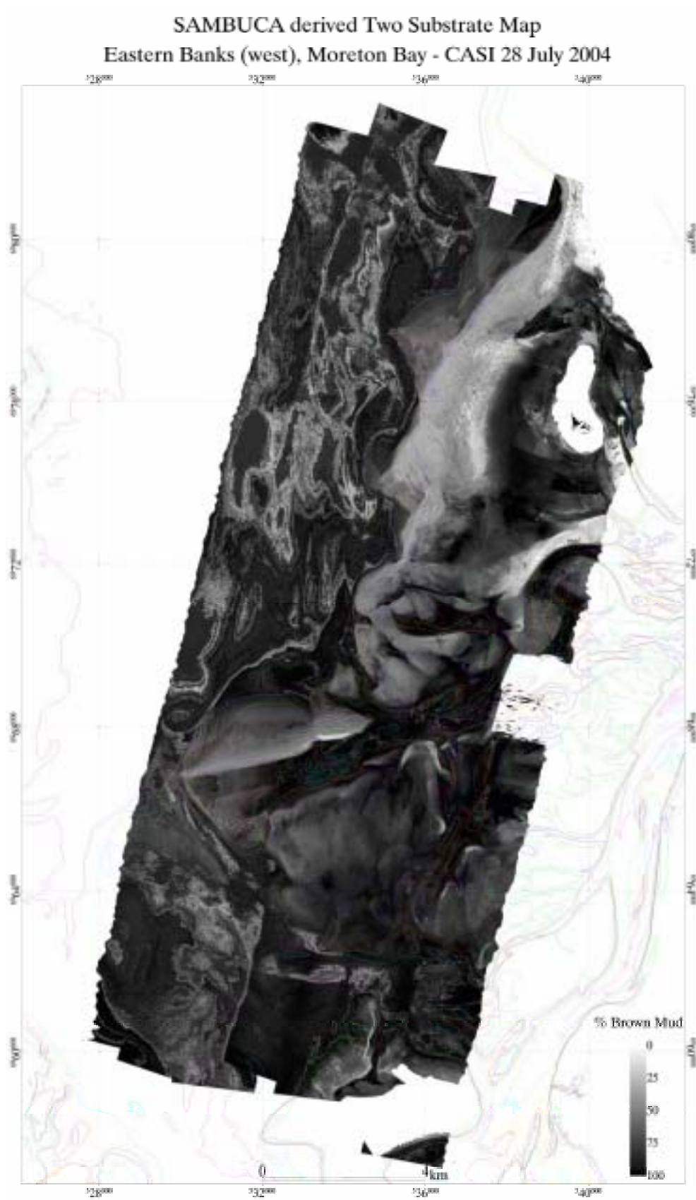
Figure 33. Benthic cover fractions and benthic cover maps for the western portion of Eastern Banks, derived from CASI-2 image using a two-substrate library (brown mud and white sand)
