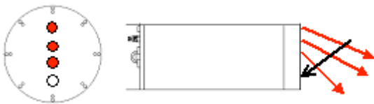
Figure 5.19. Conceptual diagram of the sensor head (left) and cross section (right) of the WET Labs ECOvsf showing the three light emitting diodes (red) and the single detector (black). The three LEDs emit light at three different angles relative to the sensor head and relative to the single detector leading to detection of backscattering centered at 110^\circ , 125^\circ , and 150^\circ , from top to bottom, respectively. Illustrations from the ECOvsf manual.
