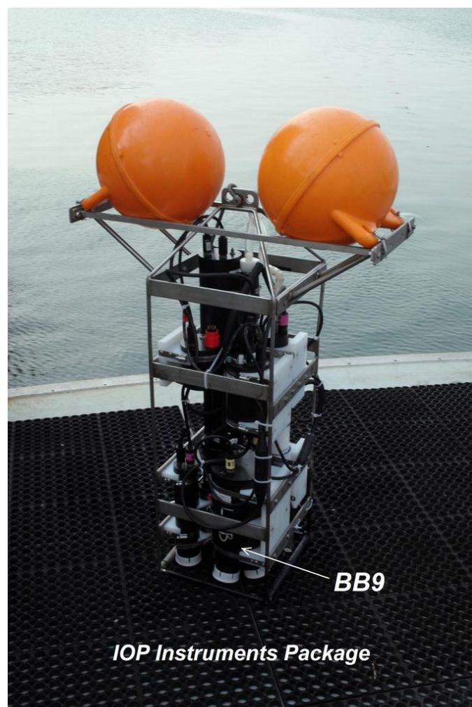
Figure 4.1. Profiling package containing the BB9. Sensor faces are pointed downward at bottom of cage.
