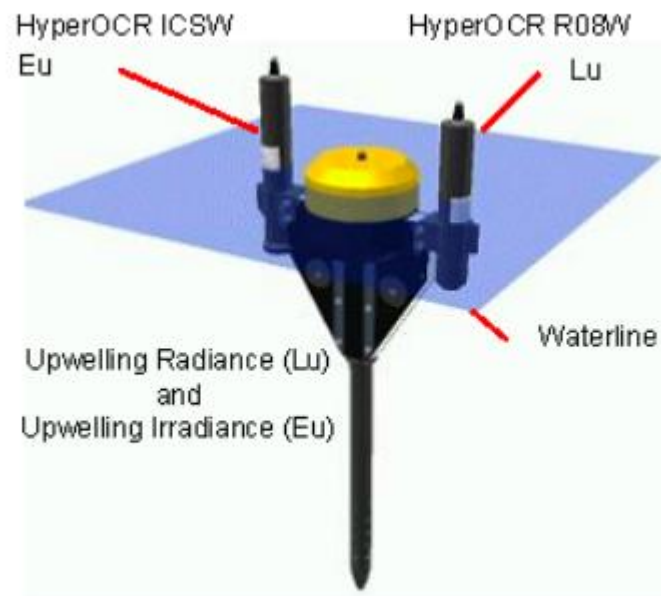
Figure 4.1. Diagram of HyperPro set-up for operation in buoy mode (Operation Manual For: Profiler II Document Number: SAT-DN-00223 Rev I, available from the Manufacturer's website)
