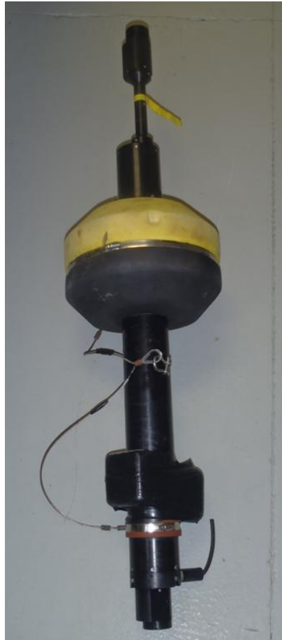
Figure 3.1 Satlantic HTSRB (owned by the Darling Marine Center, University of Maine). Note the yellow buoy responsible to stabilize the instrument and to avoid shadowing of the sensor under water. Ed sensor is located on the top, Lu sensor is located on the bottom.
