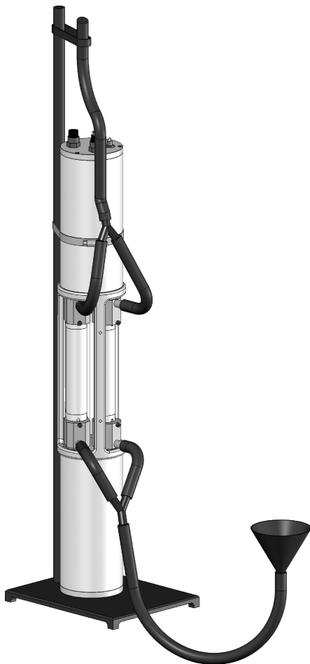
Fig. 2. Illustration of the AC-S bench-top setup used in salinity experiments.
