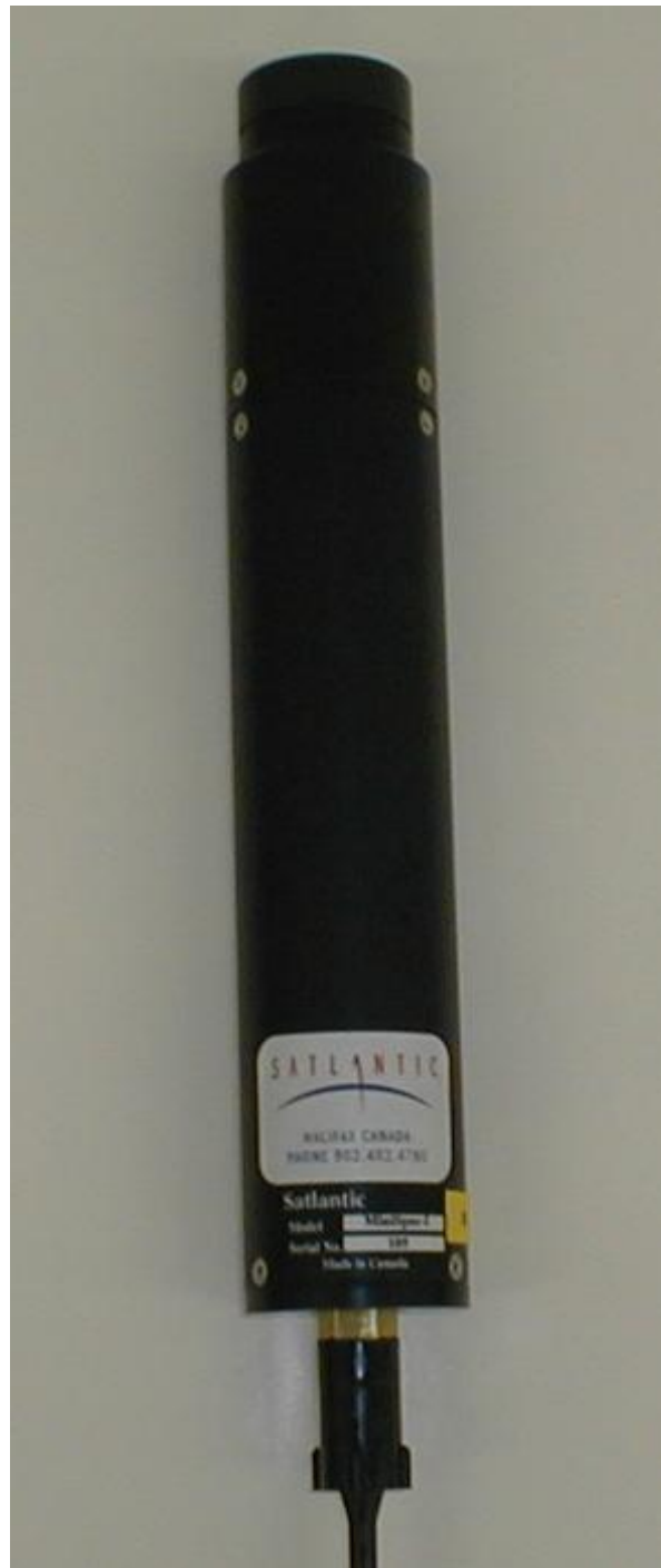
Figure A-2 – HyperOCR-I (in air) - Irradiance Configuration
