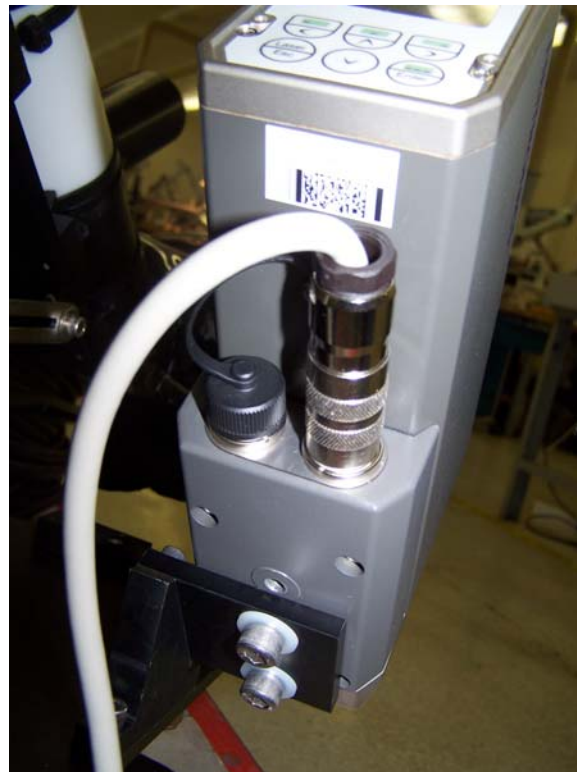
Figure D-4: Attaching pyrometer to plate
