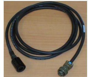
Deck Unit to 9plus test cable
