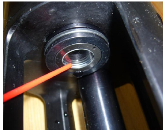
Canned air used to dry optical window (C-Rover/ac-s)
