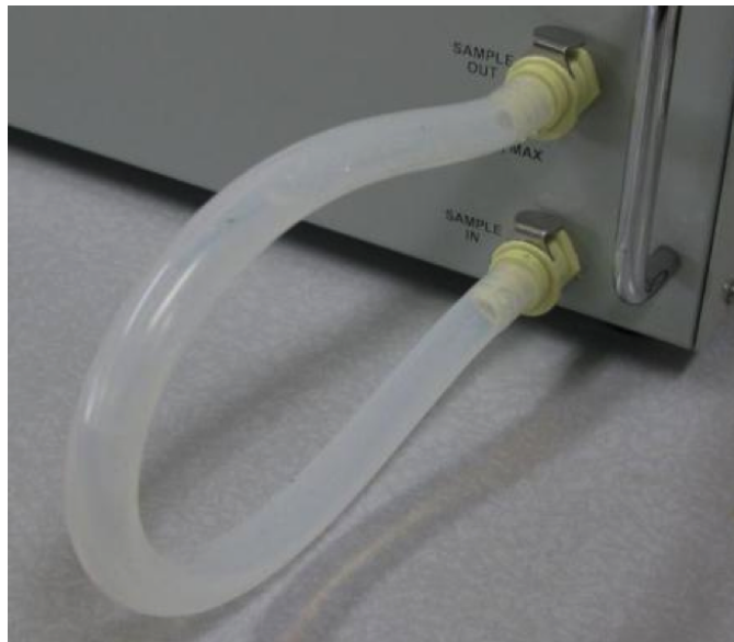
Figure 6: Input and output ports connected with a short piece of tubing prior to shipment
