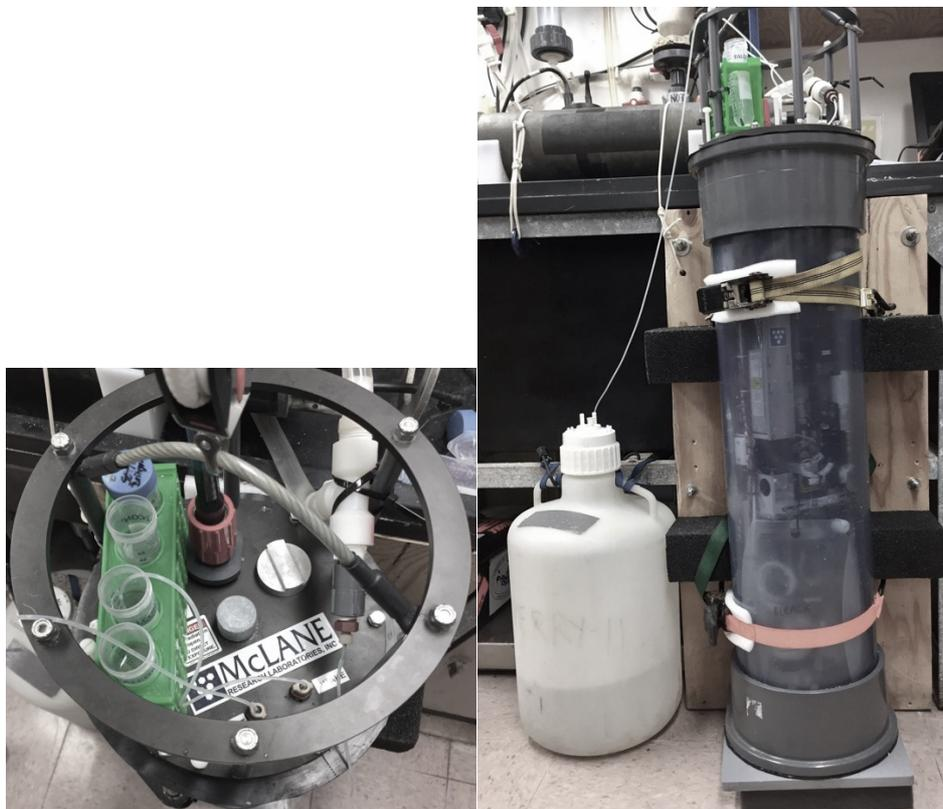
Picture 1. IFCB setup inline on the R/V Atlantis during NAAMES III
