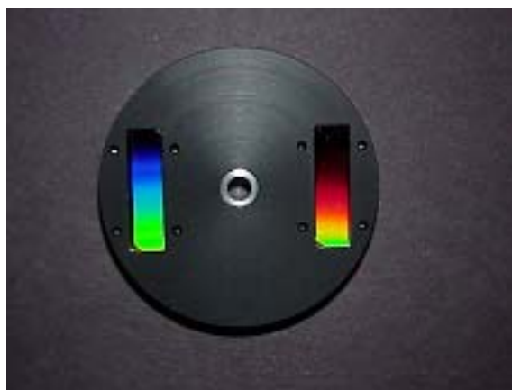
Figure 6. ac-s filter wheel
