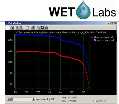
The spectral plot window shows a given spectrum vs. wavelength. The Line Number lists where it occurs in the file. You can choose which line to view by moving this slider. If you have loaded a CTD file, the temperature and salinity are also listed.
