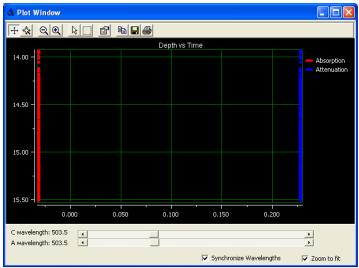
Use the sliders to change the wavelengths displayed in the depth and time plot windows. If Synchronize Wavelengths is checked, both sliders will move together, keeping the two wavelengths as close as reasonably possible. If you uncheck Synchronize Wavelengths, the sliders can be moved independently.
