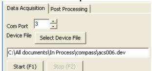
Com Port: Select the appropriate port for PC-to-meter communication.
