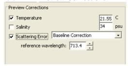
Temperature: Applies a standard temperature correction. This requires the factory calibration temperature, which should be in the dev file. It is also on the meter's data calibration sheet.
