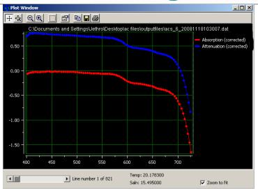
The spectral plot window shows a given spectrum vs. wavelength. The Line Number lists where it occurs in the file. You can choose which line to view by moving this slider. If you have loaded a CTD file, the temperature and salinity are also listed.
