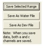
Save Selected Range brings up a dialog box that allows you to save a selected number of lines of data, corrected as per the boxes on the "Post Processing" tab, in the Compass format, cropped down to the range selected.
