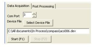
8. Click the Start button (or F1) to start data acquisition. A dialog box prompting you to save the file will appear. A default file name is automatically supplied. It indicates meter type, meter serial number, date, and time. If you do not wish to save the data, click Cancel.
