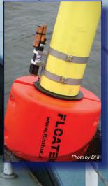
WQM upon recovery; significant bio-fouling along instrument but clear optical window from use of Bio-wiper™
