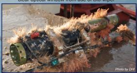
SBE 16plus V2 SeaCAT CTDs with WET Labs ECO-NTU & ECO-PAR with Bio-wiper™
