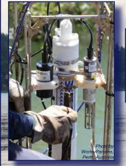
WQM-Dredges with Inductive Modem Modules & battery packs
