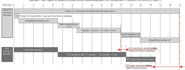
Example -- SBE 16plus V2 (Quartz Pressure sensor, ParosIntegration=2.0, PumpMode=1, NCycles=18) with ECO (\$pkt 7)
