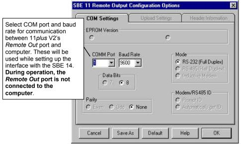
Enter the desired COM port and baud rate and click OK or Save As to save the settings when done.
